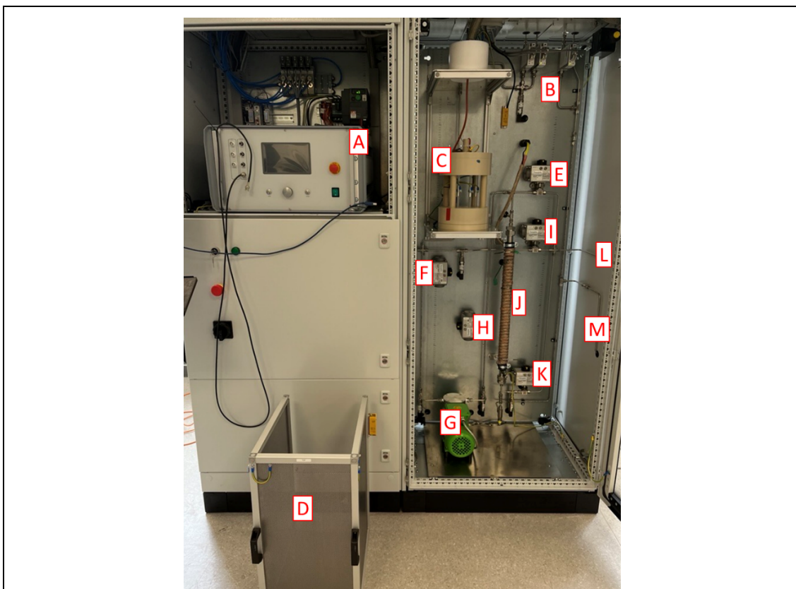
Figure 1: The pilot scale reactor set-up with its components: plasma generator (A), mass flow controllers for gases N_2 H_2 and air (B), plasma reactor (C), faradaic cage (D), valve from plasma reactor to analysis unit (E), valve from plasma reactor to vacuum pump (F), vacuum pump (G), valve from vacuum pump to sorption unit (H), valve from pump to analysis unit (I), sorption unit (J), valve from sorption unit to analysis unit (K), sample gas to analysis unit (L), sample gas from analysis unit to exhaust (M).
