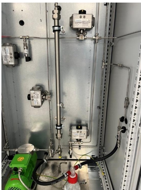
Figure 1. Summary of the experimental set-up with the sorption unit, water trap and mass flow controllers (not pictured).
