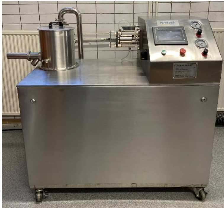
Figure 6. Extruder at HB production with capacity for 3kg/batch.
